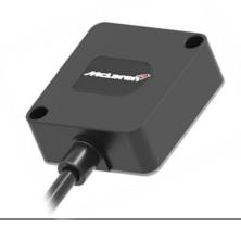
These sensors provide three axes angular rate measurements in a single robust package. The sensors filter the data and output the measurement via three linear 0-5 volt outputs.
