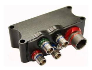
The HIU-3 is a local, micro-processor controlled sensor interface unit. It is small and light, designed to be mounted on the wheel hub, thus reducing the harnessing on the car. The unit can withstand the high radiated temperatures from the brakes whilst the car is stationary and the vibration from the wheels whilst the car is moving.
