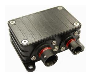
The LIU-4 provides signal conditioning for four 5 wire LVDT positioning sensors. When the LVDT sensors are being used in latency critical control systems, the conditioned signals are passed to the host ECU as four 0 to 5V analogue outputs. Where LVDT sensors are used for diagnostics or where control system speed is less critical, the signal conditioned values can be made available over the CAN bus communications link in order to reduce system harnessing.
